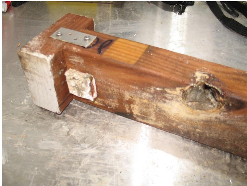
Figure 10: Mould growth on the surface of a boron treated radiata pine sample after twelve months exposure (sample 601).
