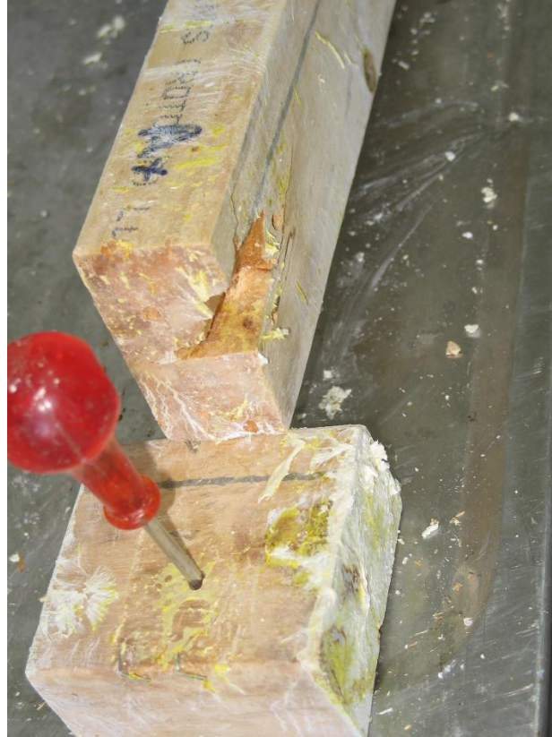
Figure 13: Decay in the joint of an untreated radiata pine sample after six months exposure (sample U10).
