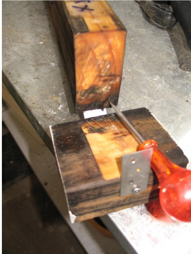
Figure 9: Suspected soft rot on the bottom edge of a boron treated radiata pine sample after twelve months exposure (sample 604).
