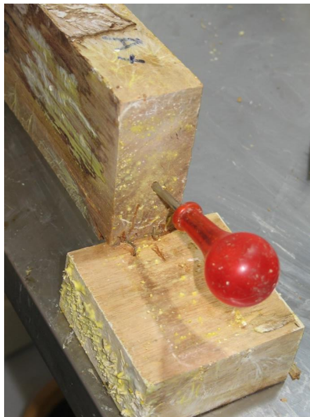
Figure 8: Decay in the joint of a Eucalyptus regnans sample after twelve months exposure (sample 408).
