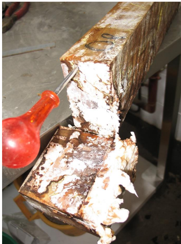
Figure 4: Decay in the joint of a heartwood Cupressus lusitanica sample after twelve months exposure (sample 235).
