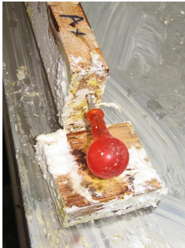
Figure 6: Decay in the joint of a Douglas fir sample after twelve months exposure (sample 503).
