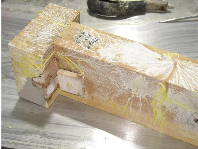
Figure 7: Mycelium growth on the surface of a Eucalyptus regnans sample after twelve months exposure (sample 409).
