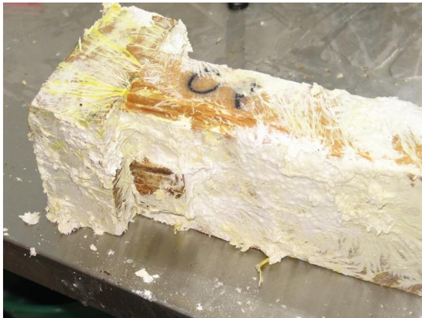
Figure 2: Mycelium growth on the surface of a Cupressus lusitanica sample after twelve months exposure (sample 206).
