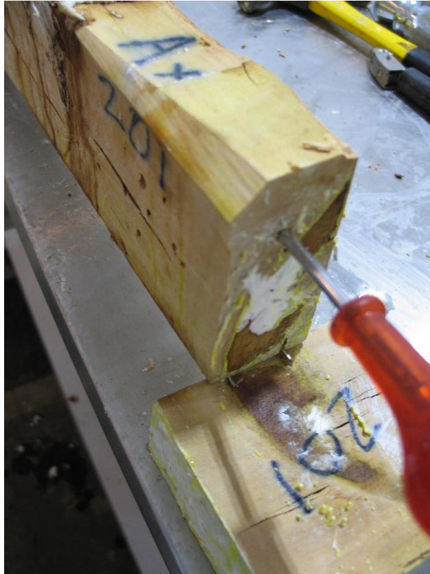
Figure 3: Decay on the surface and in the joint of a mixed heartwood\sapwood Cupressus lusitanica sample after twelve months exposure (sample 201).
