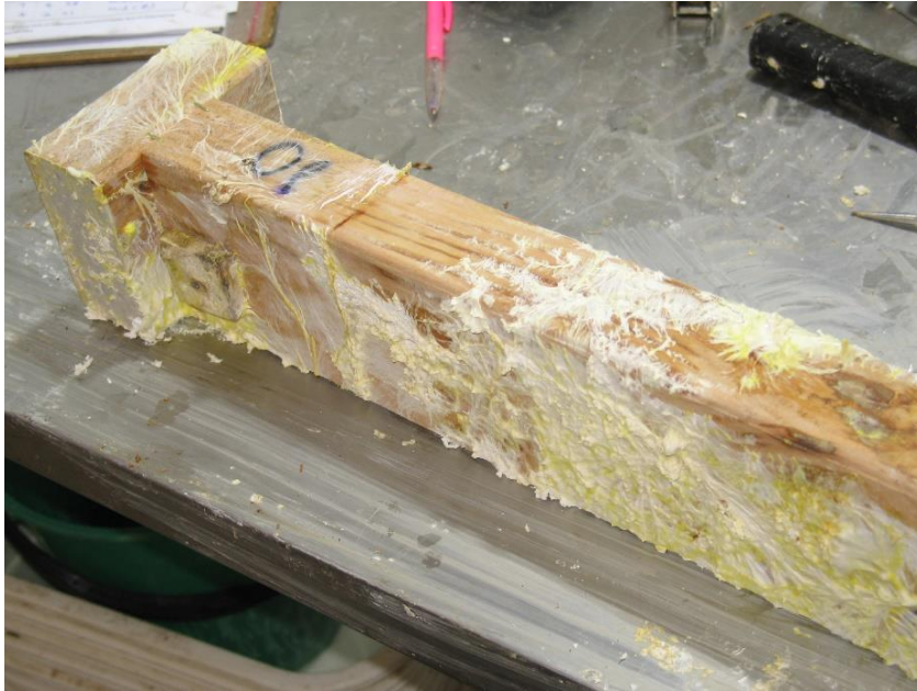
Figure 5: Mycelium growth on the surface of a Douglas fir sample after twelve months exposure (sample 502).
