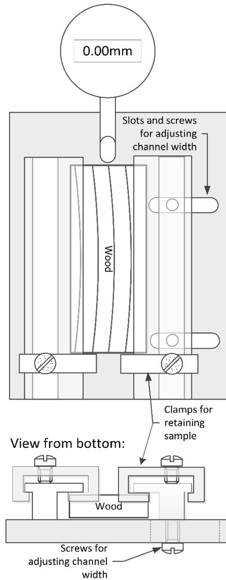
Figure 1. Front and bottom views of Swellometer jig.
