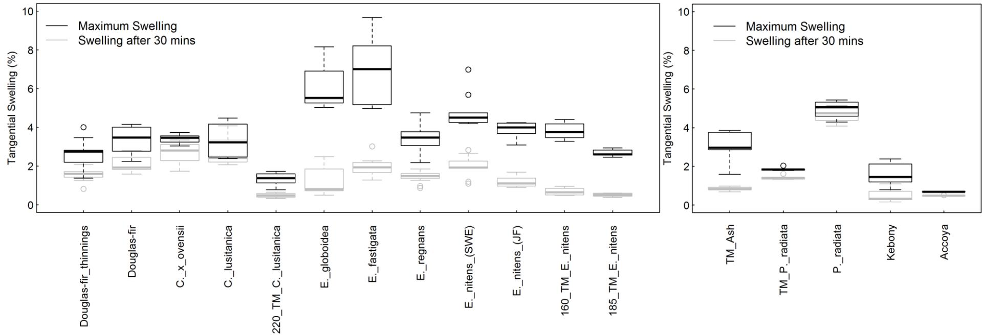
Figure 3. Swelling after 30 minutes (grey boxes) and 3 days (black boxes) of water soaking. The left hand panel shows SWP species (including thermal modifications), the right hand panel shows commercial benchmarks.
