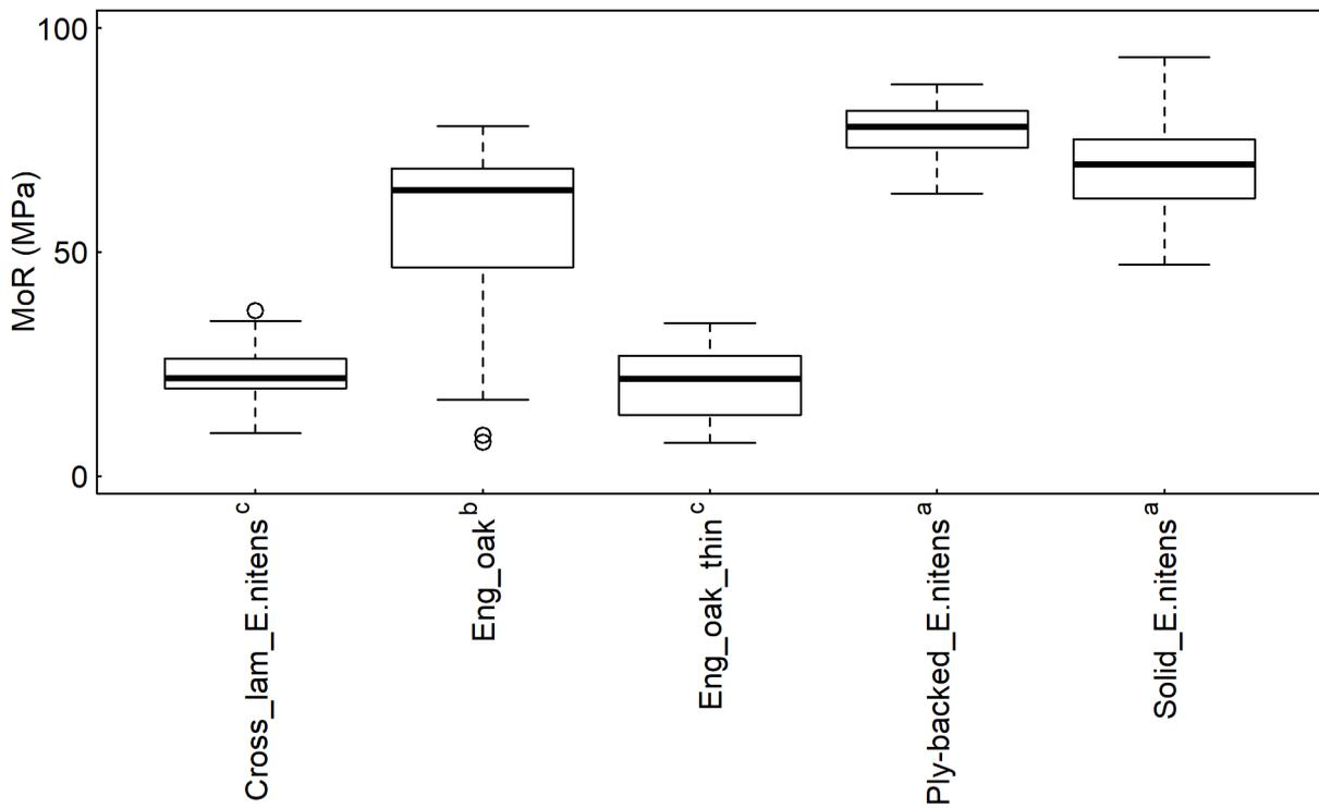
**Figure 11.** Modulus of rupture (MOR) of different flooring types. Superscript letters indicate treatments that are not significantly different (95% confidence level).
