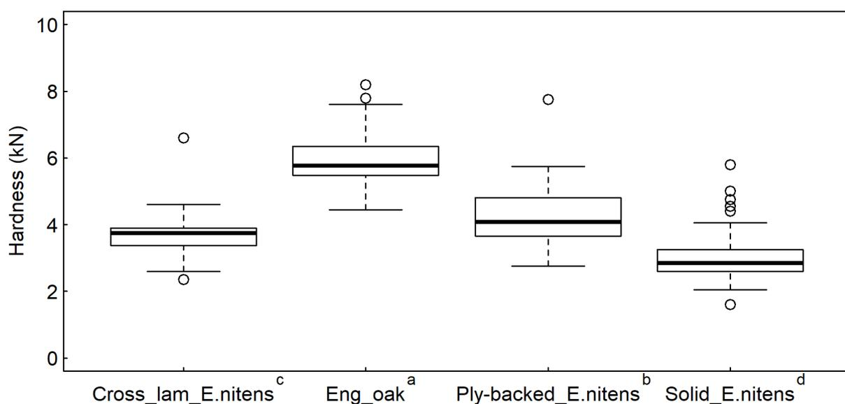
**Figure 8.** Hardness of the top face of each flooring type. Superscript letters indicate treatments that are not significantly different (95% confidence level).
