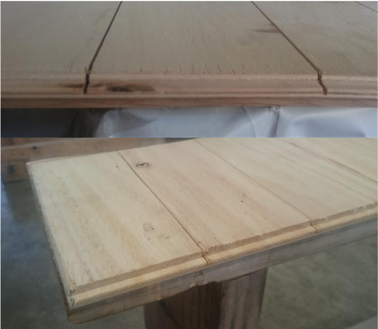
**Figure 10.** Back faces of the thin engineered oak (top) and cross-laminated *E. nitens* (bottom). Both views are of the board edge.
