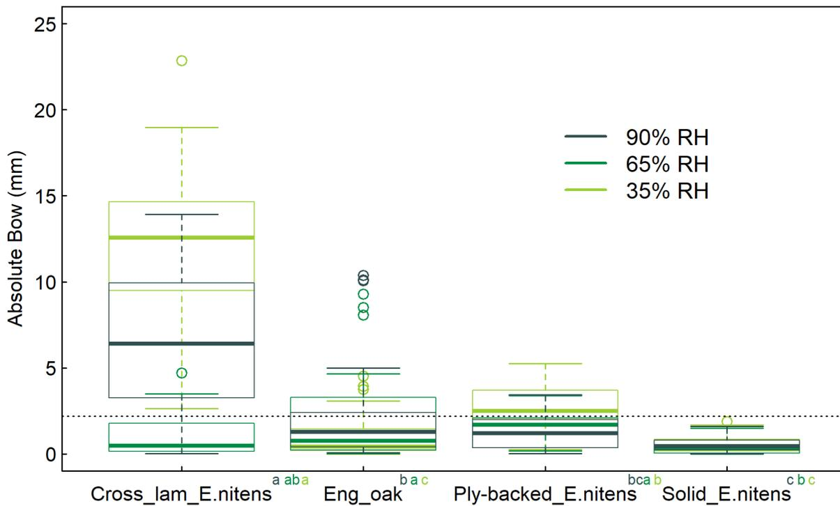
**Figure 4.** Levels of bow at each moisture content for each board type. Superscript letters indicate groups that are not significantly different to each other (95% confidence level) the text colour of the letters indicates the humidity condition they apply to (as per the figure legend). The dotted line shows the maximum bow allowed in the Australian Standard *at the time of installation*.
