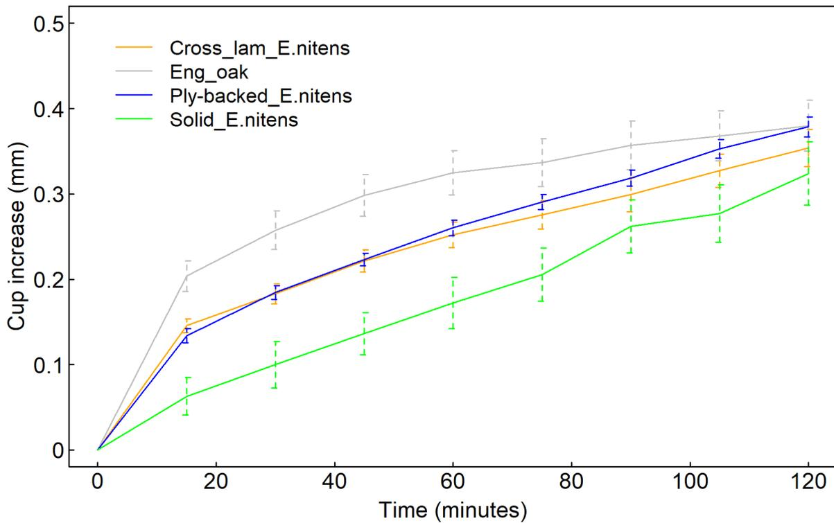
**Figure 5.** Increases in cup over time for each board type. Error bars indicate one standard error.
