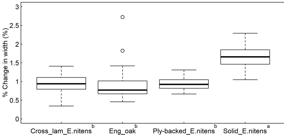
**Figure 1.** Change in width between 35 and 90% RH conditions for each board type. Superscript letters indicate groups that are not significantly different to each other (95% confidence level)
