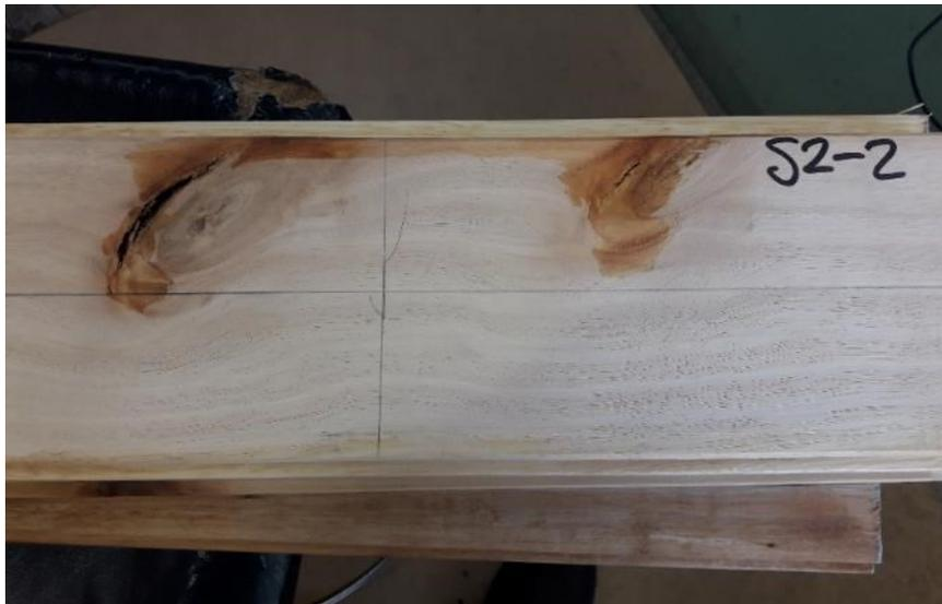
**Figure 6.** Water wicking through a knot to the top face of a solid *E. nitens* board after the lower face was submerged in water
