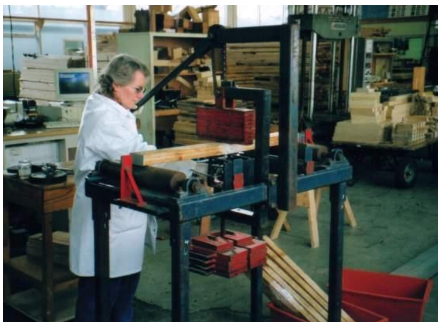
Figure 14: Stiffness testing assembly
