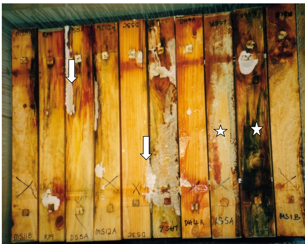
Figure 9: After twenty-four weeks' exposure. Decay developing on Douglas-fir (arrows) and Lawson cypress sapwood (stars)
