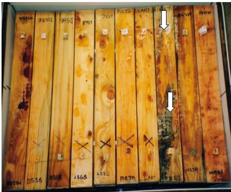
Figure 8: After four weeks' exposure. Sapstain and mould developing on Lawson cypress sapwood samples (arrowed).
