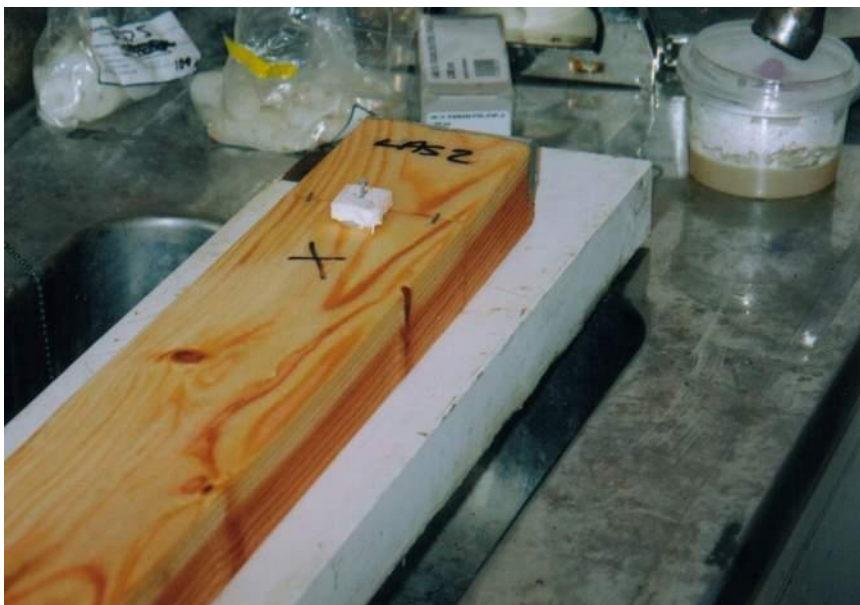
Figure 7: Larch sapwood sample before exposure. Decay inoculum attached at joint
