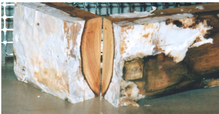
Figure 4 – Sample MS12A, Layer 6, Tank 2 after 52 weeks exposure. Macrocarpa sapwood sample showing severe Auckland brown rot decay in the sapwood stopping abruptly at the heartwood boundary.
