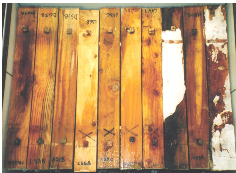
Figure 8 – Layer 7 (Top layer) in Tank 1 after 52 weeks exposure. The sample at the right hand end is M15AH, macrocarpa heartwood. Although there was extensive Auckland brown rot mycelium on the surface, spreading from the sample underneath, there was only minor decay associated with it. The other sample with extensive mycelium on it, LS1B (Lawson cypress sapwood) was badly stained but contained very little decay.
