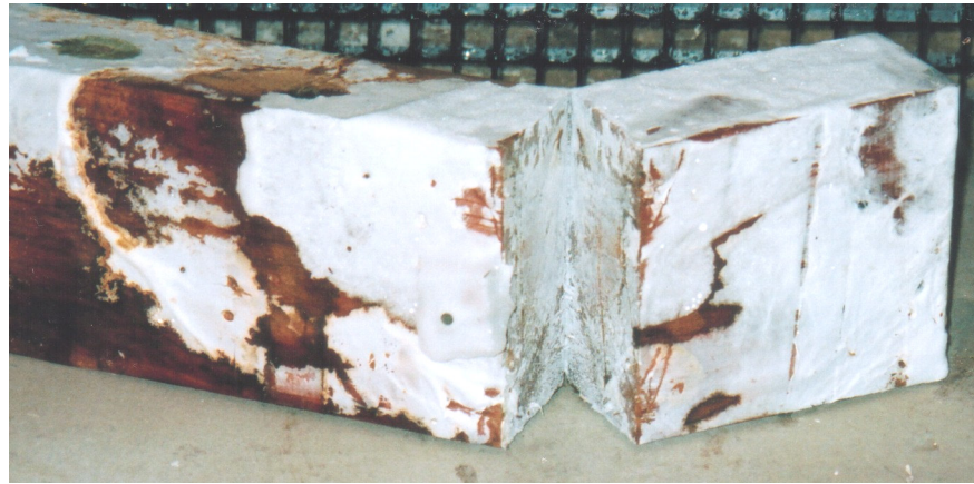
Figure 9 – Sample M15AH, Layer 7, Tank 1 after 52 weeks exposure. Extensive Auckland brown rot mycelium on the surface and through the joint of a macrocarpa heartwood sample but only small patches of lightly established decay.
