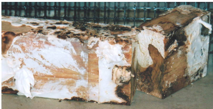
Figure 5 – Sample LH6A, Layer 5, Tank 2 after 52 weeks exposure. This Lawson cypress heartwood sample was severely stained and largely covered by Auckland brown rot mycelium. Although there was minor patch of decay in the joint the sample was otherwise sound.
