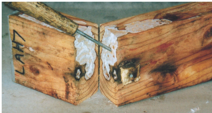
Figure 10 – Sample LAH7 (Larch heartwood), Layer 7, Tank 1 after 52 weeks exposure. There was a small amount of Auckland brown rot mycelium and minor decay on one edge but moderate-severe decay in the joint. Extensive mycelium on the adjacent Lawson cypress sapwood sample, LS1B, appeared to have spread from sample LAH7 but had not caused any significant decay in the Lawson cypress.
