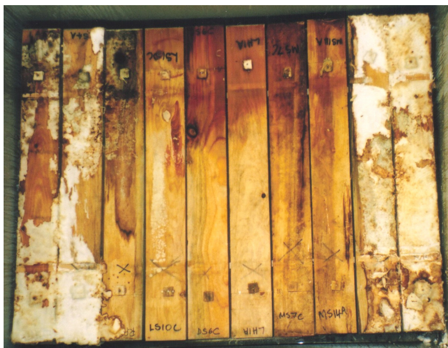
Figure 7 – Layer 2 (2 nd from bottom) Tank 2, after 52 weeks exposure. Five samples, Larch sapwood, Larch heartwood, Lawson cypress sapwood and radiata pine have extensive Auckland brown rot mycelium on them and this has spread between samples. All contained moderate-severe decay. Sample LS10C is a boron treated Lawson cypress sample with extensive pale coloured mould on the surface but no decay.
