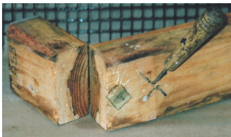
Figure 6 – Sample LAS3, Layer 4, Tank 2 after 52 weeks exposure. Larch sapwood sample with severe decay extending through the sapwood and into the heartwood. This decay is typical of Antrodia xantha , with very little visible mycelium on the surface even when the wood is severely decayed.
