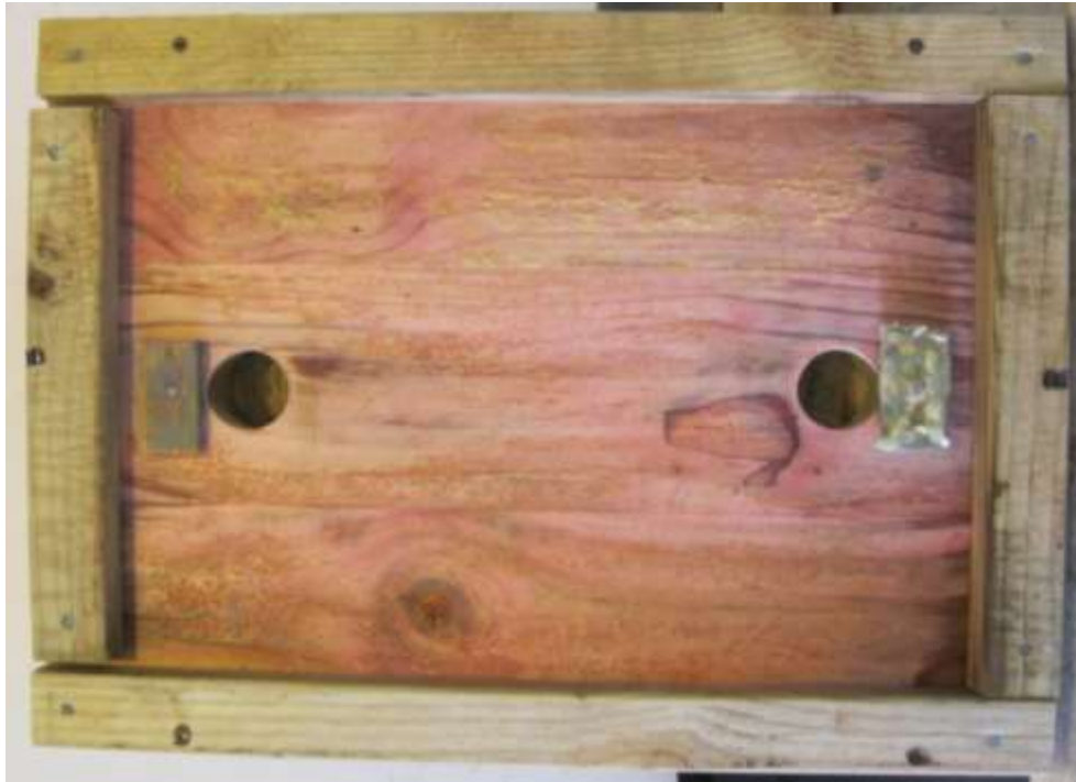
Figure 9 – Treated, unleached assembly T2 after 28 weeks exposure. There was no decay mycelium from the feeder blocks but there was extensive mould on the surface and the feeder blocks.
