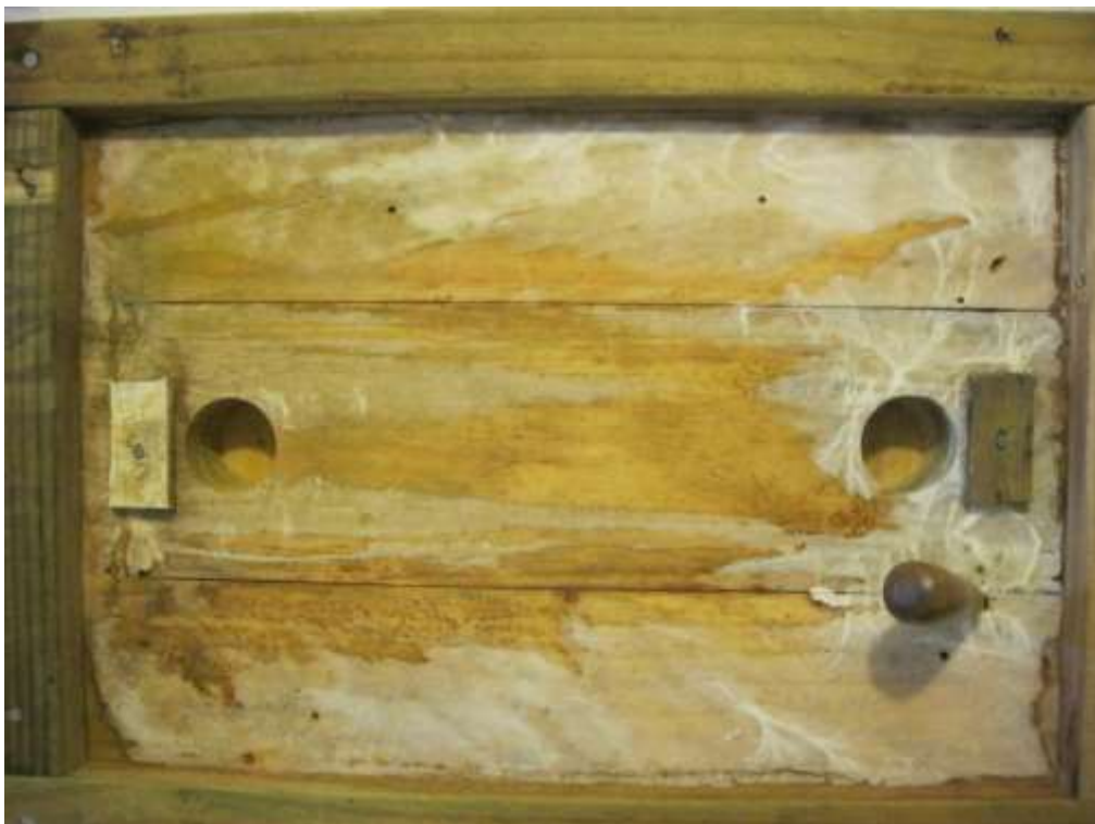
Figure 10 – The face of untreated unit (U5) after 56 weeks in the exposure room. There was extensive decay mycelium and deep decay over the whole of the face.
