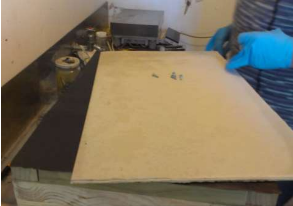
Figure 3 – Unit preparation of a CLT sample after fungal inoculation. Fibre cement panels and building paper were fixed on top of H3.2 treated CCA battens on each side of the sample.
