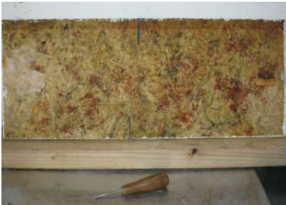
Figure 4 – A. xantha decay feeder block near the right end on the reverse of a leached NZSB sample SL8 after six weeks exposure. There was no mycelium development from the feeder block but mycelium from the O. placenta feeder block on the other side of the sample had penetrated the sample towards the left end. There were extensive moulds over the whole of the sample.
