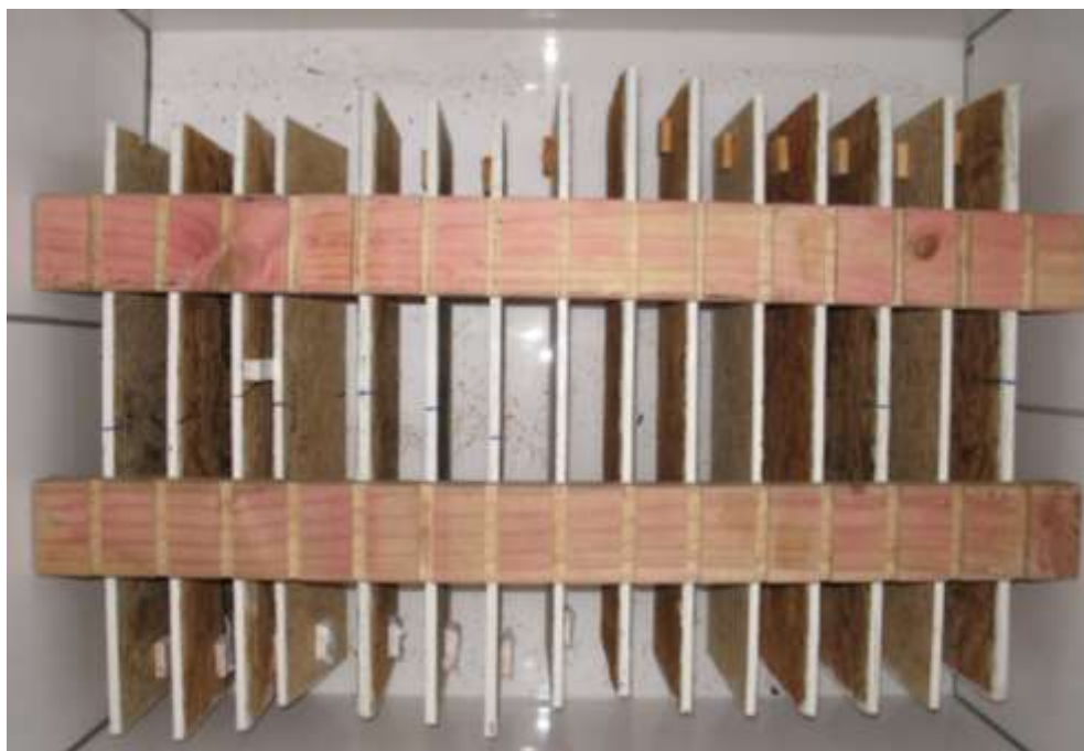
Figure 1 – Samples of OSB in slotted bearers in the exposure tanks. The O. placenta feeder blocks were on one face at one end of the samples, the A. xantha feeder blocks were on the reverse side at the other end.
