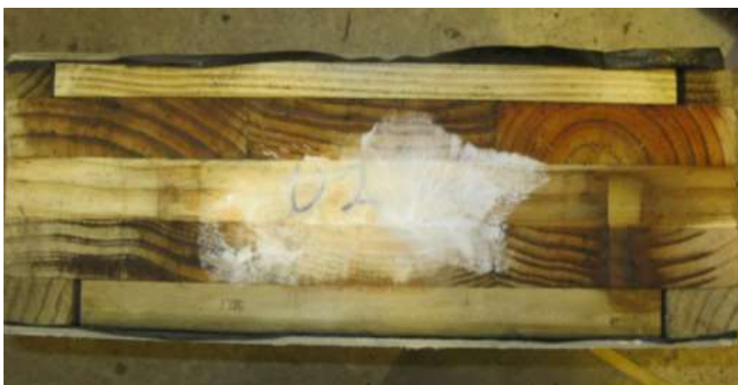
Figure 7 – The lower end of untreated unit (U2) after 12 weeks in the exposure room. The mycelium from the O. placenta feeder block had penetrated under the treated batten and was developing on the outer surface of the assembly.
