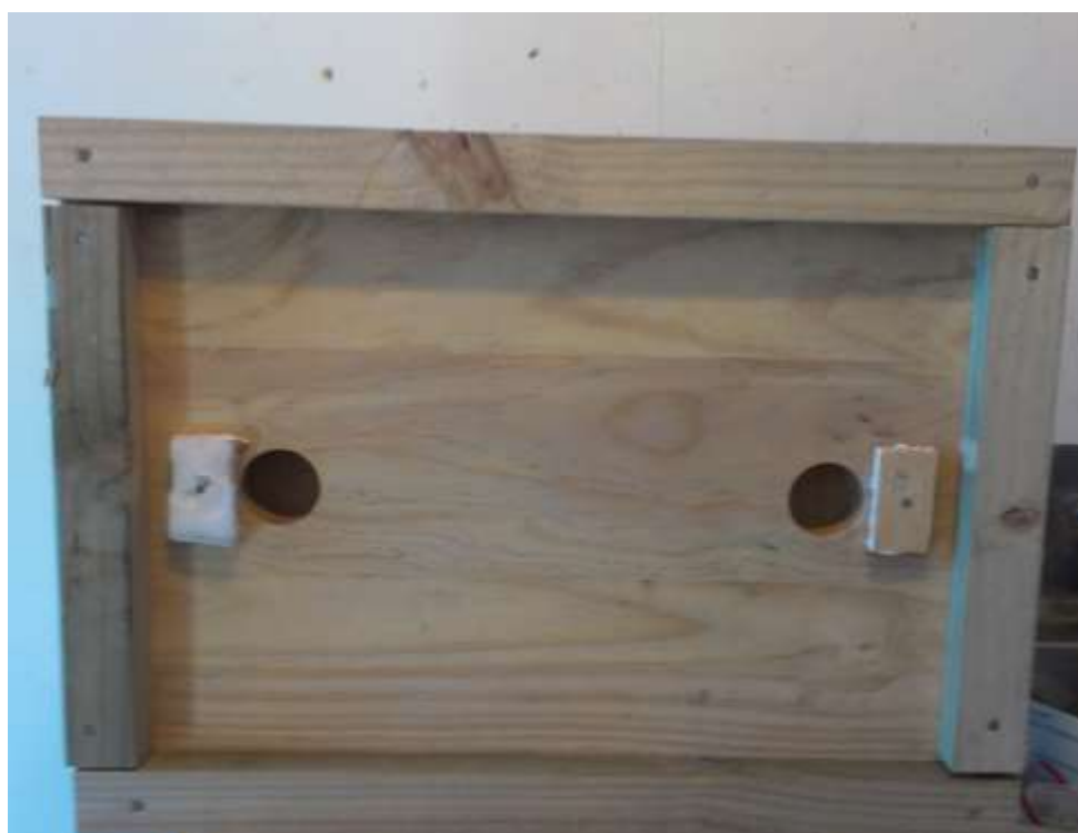
Figure 2 – A sample of CLT showing fungal inoculum of O. placenta and A. xantha at the opposite end close to 50 mm diameter holes that were bored after treatment.
