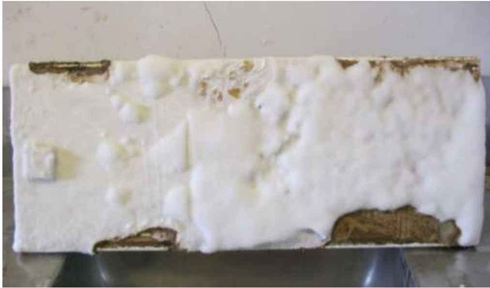
Figure 5 – Widespread O. placenta mycelium covering the reverse of sample SO3, imported OSB which had not been leached, after 26 weeks exposure. The mycelium had completely covered the A. xantha feeder block. There was no mycelium or decay in the areas immediately adjacent to where the sample was in contact with the boron treated bearers
