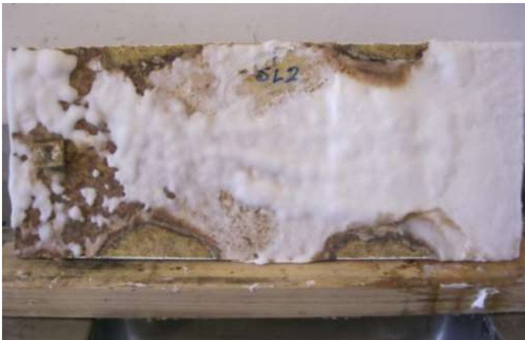
Figure 6 - Widespread O. placenta mycelium covering the face of sample SL2, NZSB which had been leached before exposure, after 26 weeks exposure. The mycelium around the feeder block had degenerated since the 14-week assessment. Severe decay was present throughout the board, except close to the bearers.
