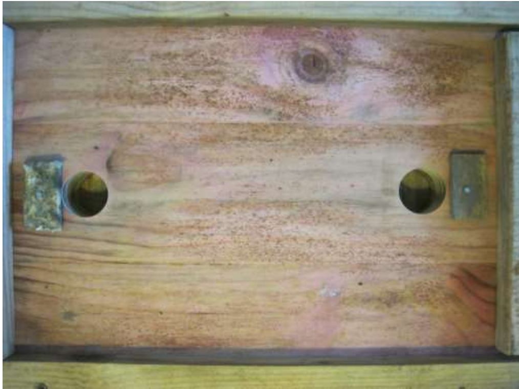
Figure 11 – The face of treated (not leached) unit (T2) after 56 weeks in the exposure room. There was no decay but there was extensive mould across the face and on the decay feeder blocks.
