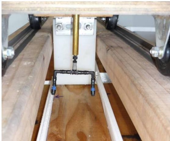
Figure 6. Spray nozzles directing water onto timber surface and timber edge in contact with building underlay material
