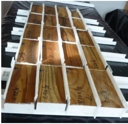
Figure 4. Set up on specimen boards on PVC plates. (View is of final sub-sample of each board before trial was terminated)
