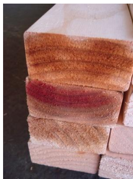
Figure 1. PVC heart/sapwood test; top board is sapwood and red colour on second board identifies presence of heartwood
