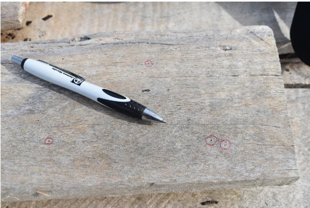
Figure: 12 – In contrast to the tōtara, an adjacent stack of taraire timber, milled at the same time, has been damaged by the common household borer ( Anobium punctatum ), despite being sprayed with Clear-Metalex & Turps.
