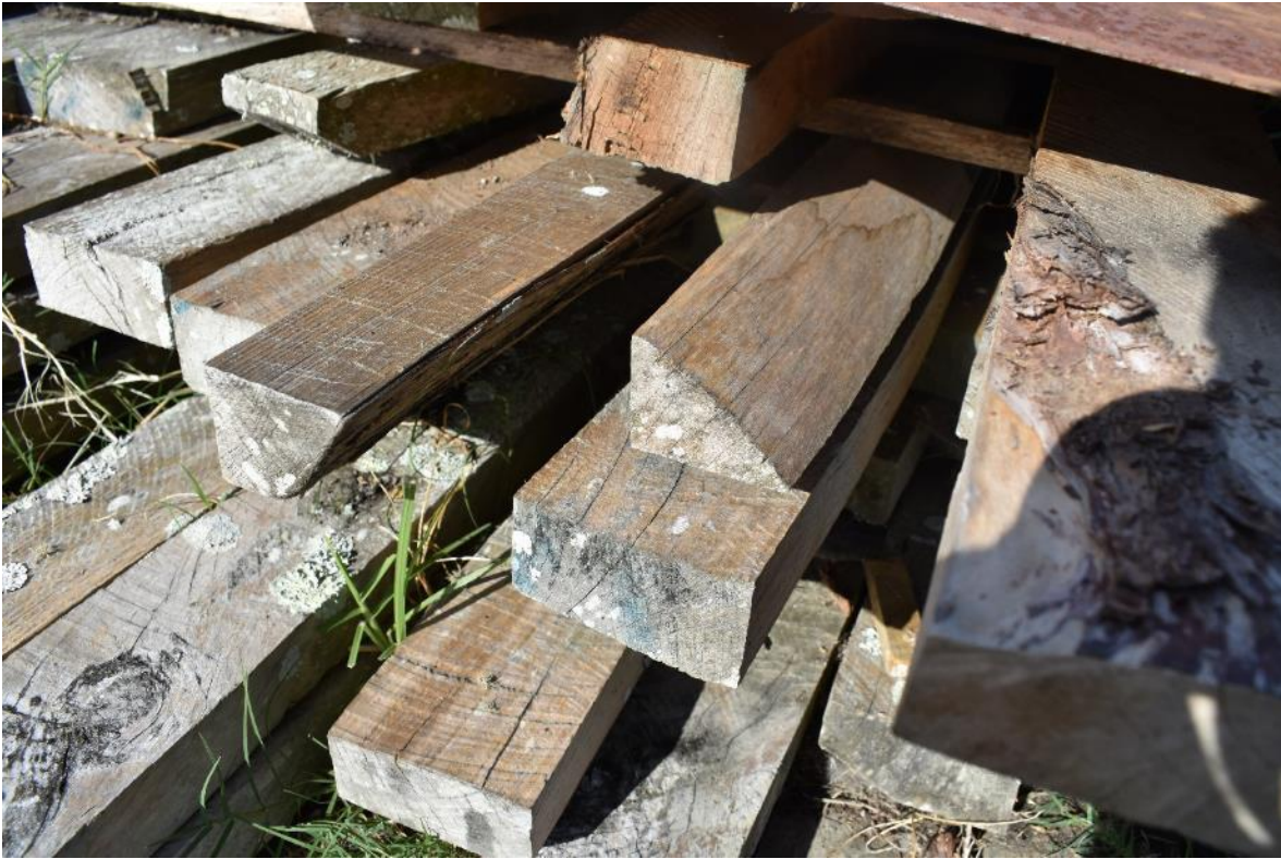
Figure: 11 – No incidence of borer was observed in the stack of untreated tōtara timber, which includes boards that clearly comprise a high proportion of sapwood timber.
