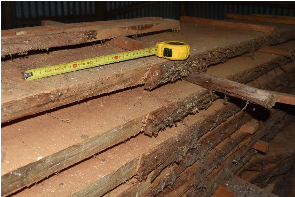
Figure: 5 – No evidence of borer damage was observed on any of the tōtara slabs or sawn lumber stored for over 7 ½ years in the same shed as the kauri slabs that were infested with borer.
