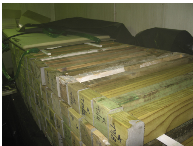
Fig. 2. “I” samples in an exposure stack. The decay feeder blocks visible on the right were O. placenta . The feeder blocks at the left end were on the reverse face and were infected with A. xantha .
