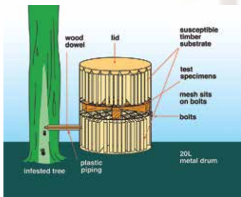
Figure 3. Field exposure to subterranean termites using the drum technique.
