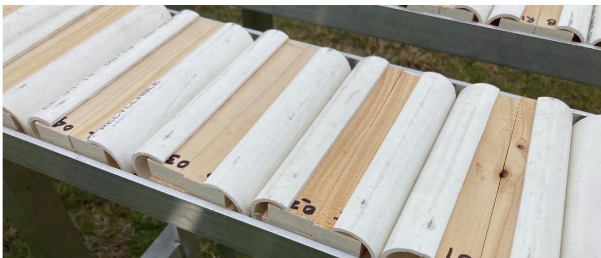
Figure 1: Installed lap joints showing narrow faces exposed at the surface with wide faces below.
